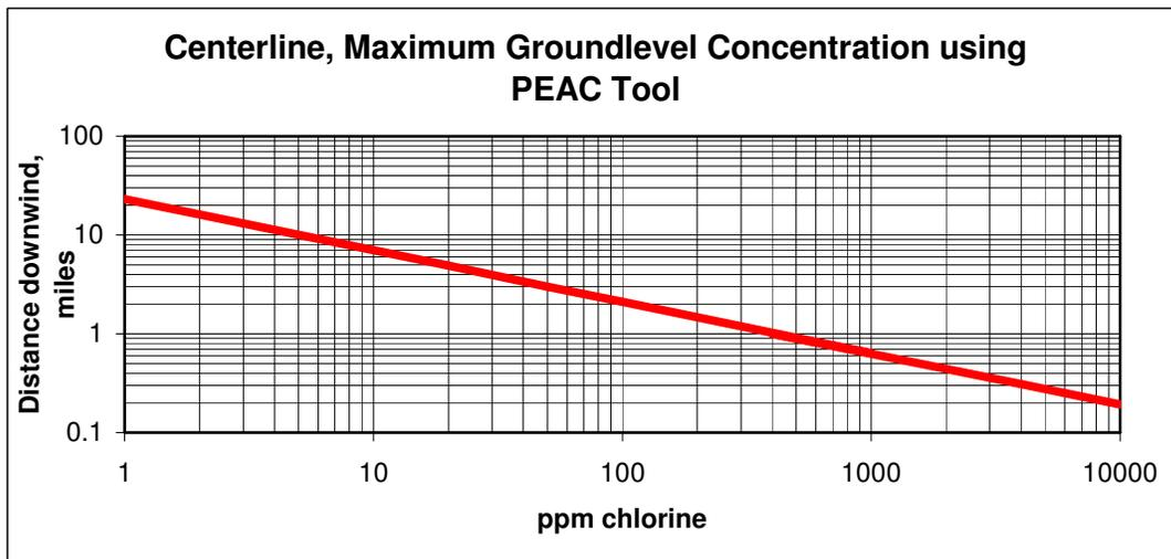
The Hanna paper using the SCIPUFF model predicted a maximum 1750 ppm chlorine concentration at a distance of 1 km downwind. The PEAC tool using a 35,700 lb instantaneous release predicted a downwind distance of 0.5 miles corresponding to 1750 ppm
