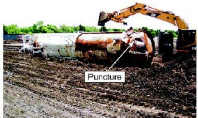
Damaged Chlorine Railcar, photo taken during cleanup operations, from Railroad Accident Report.
